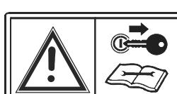
Pull the ignition plug out before maintenance and repair work.
